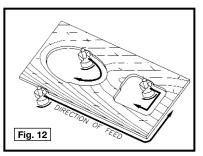
When making cuts on all four edges of the workpiece, make the first cut on the end of the piece across the grain. Thus, if chipping of wood occurs at the end of a cut, it can be removed when making the next cut parallel with the grain.
